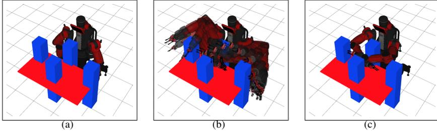
Fig. 10: The initial (a) and goal (c) configuration, along with the path (b) used in the experiments with the Baxter. The table is indicated with red, and the four pillars are indicated with blue.
