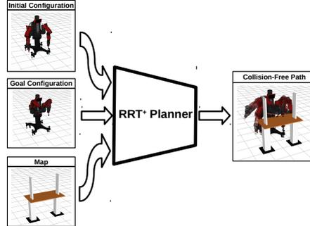
Fig. 3: An overview of the usage of the proposed planners. The initial and goal configurations along with a map, shown on the left, are the inputs that the  $RRT^+$  planners utilize to produce a collision free path, shown on the right.
