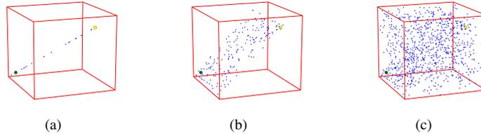
Fig. 2: Sampling in one, two and three dimensions in  $\mathcal{C}$ . Red lines indicate the boundaries of  $\mathcal{C}$ , the yellow dots indicates  $q_{init}$ , and the green dots indicate  $q_{goal}$ .
