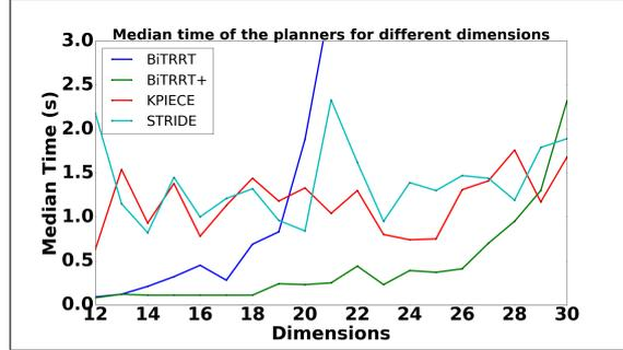
Fig. 7: Comparison of the median time for the Cluttered Random environment from 12 to 30 dimensions of BiT-RRT and BiT-RRT<sup>+</sup>, KPIECE and STRIDE. Interestingly, BiT-RRT<sup>+</sup> is more than 200 times faster than BiT-RRT for 30 DoF.
