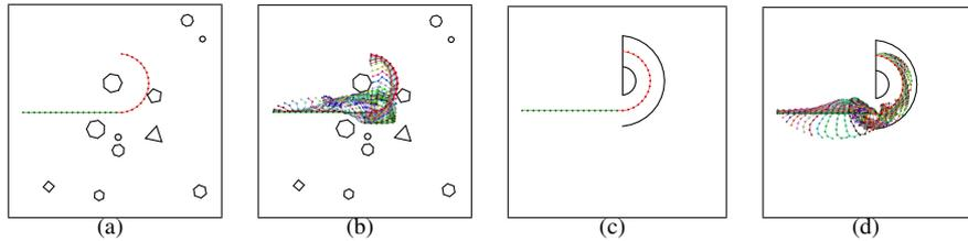
Fig. 4: The two different environments, called Random Cluttered and Horn [11]. In (a) and (c) the two planning problems are presented. The red chain indicates the initial configuration ( $q_{init}$ ) and the green chain represents the goal configuration ( $q_{goal}$ ). In (b) and (d), solutions for the two environments, produced by RRT<sup>+</sup>-Connect, are shown using a random color-palette.
