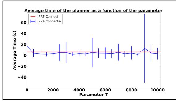
Fig. 9: Sensitivity to  $T$  from 0 to 10000 with step 500, given  $\alpha = 1.6$  for 200 runs per value of RRT<sup>+</sup>-Connect in the Random Cluttered environment for 15 degrees of freedom.
