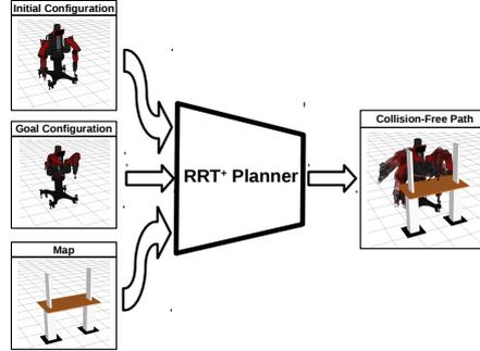
Fig. 3: An overview of the usage of the proposed planners. The initial and goal configurations along with a map, shown on the left, are the inputs that the RRT<sup>+</sup> planners utilize to produce a collision free path, shown on the right.
