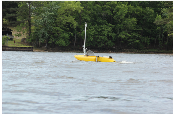
Fig. 1: AFRL Jetyak ASV collecting water quality data along trajectory at Lake Wateree, SC, USA.
