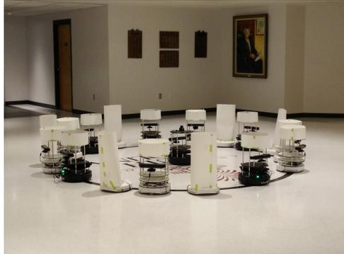
Fig. 1. The robot, a TurtleBot 2 equipped with a laser range finder surrounded by several dynamic obstacles (other robots).
