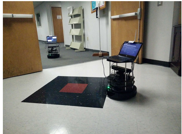
Fig. 1 TurtleBot 2 robots equipped with a WiFi dongle, deployed in the engineering building at the University of South Carolina, building a communication map
